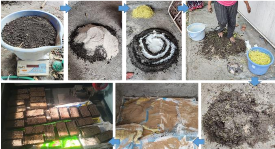
Figure 2: Process of Block Making
