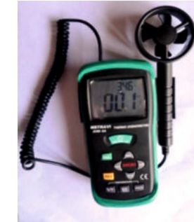
Figure 7: Anemometer to measure air speed
