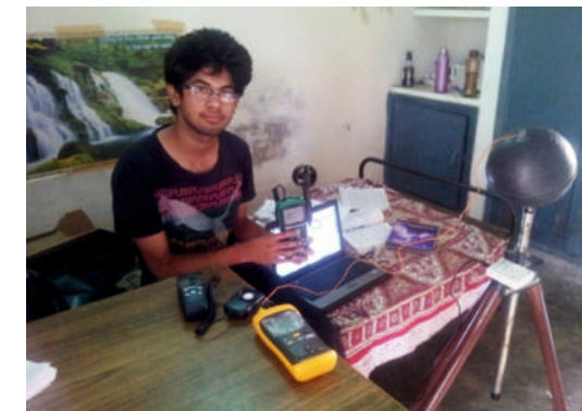
Figure 6: Typical Experimental set up using Anemometer, Lux meter, thermo couple for Globe temperature and Data logger for spot measurements.
