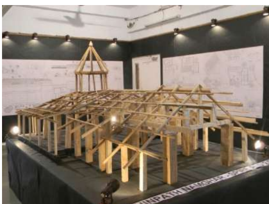
Figure 16: Model of Post and Lintel timber construction of Dokhinpat Namghar, Credit: KRVIA Students' work 2010
