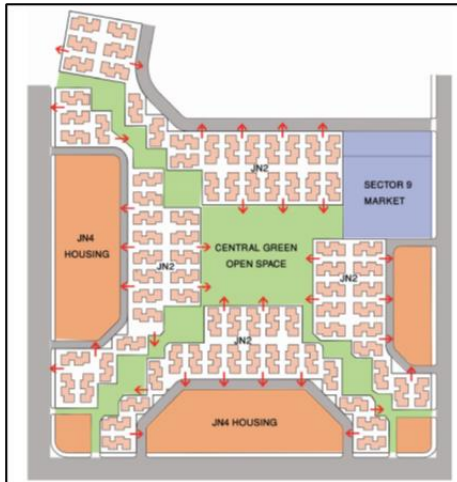
Figure 11: Plan of JN2 Housing, Sector 9, Vashi showing how multiple entry exit points facilitate an outward looking housing project connected to the city. (Source: Author)
