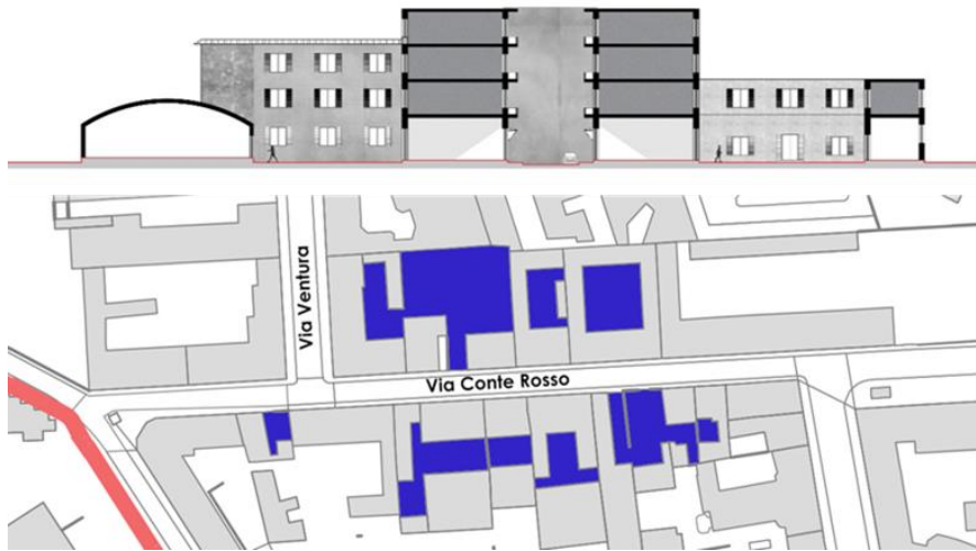
Figure 9: Section through the street indicating the openings at street level leading to the courtyard spaces and plan indicating the series of courtyards located off via Conte Rosso
