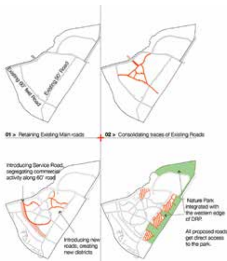
Figure 1: Master plan of Dharavi along the lines of a street based system
